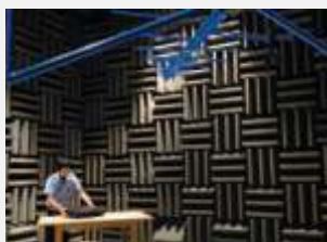
Acoustic radio wave anechoic chamber
